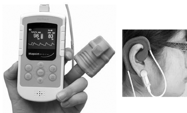
Figure 1: Pulseoxymeter used in the present study. Peripheral pulse was obtained from a sensor attached on the finger tip (left) or earlobe (right).
