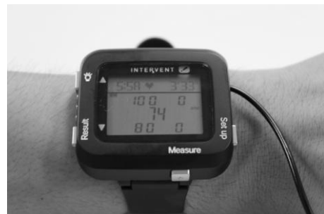
Figure 1 Pulse monitoring device (PMD) The patients could monitor their pulse rate during home exercise.
